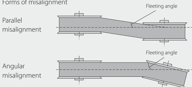
To check alignment, you will need a straight edge or, for long centre distance drives, heavy string. Line the straight edge or string along a machined face of both pulleys. Misalignment will show up as a gap between the face of the pulley and the straight edge or string. When using this method, make sure the distance between the groove edge and the outer rim of both pulleys is identical. Pulleys can also be checked for tilting with a spirit level.
