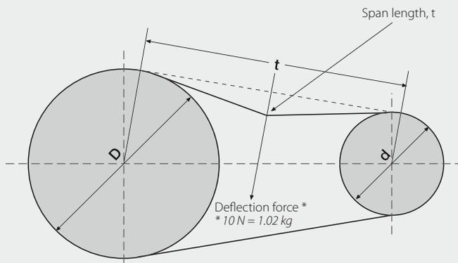
The final step is to check belt tension, and, if necessary, retension the belt. If too little tension is applied, V-belts may slip. The correct tension is the lowest tension at which the belts will transmit power when the drive is at full load.
